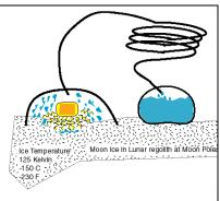
**FIGURE 3** A refrigerator-sized nuclear heater can melt and vaporize 100,000 tons ice per year. A steam rocket uses the condensed water directly as propellant.
