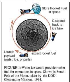
A nuclear heated steam rocket (NSR) would launch payloads from the lunar surface to low lunar orbit (LLO). The rocket would then return to the surface to launch more payloads. A separate facility located at an ice formation on the moon would use a nuclear heater to melt ice, as in Figure 3. The facility would condense pure water for the NSR to use in its rocket propellant tank.
